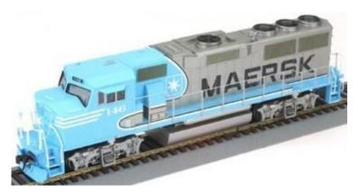
Since 2009, Athearn has provided the option of purchasing some of their models equipped with Tsunami sound. If you have a GP60B or a GP60M model without sound that you would like to upgrade, purchase SoundTraxx P.N. 885013. This board is designed to simply replace the factory PCB that supplies power to the locomotive. You can complete the installation in one to two hours with no modification required to the model!
